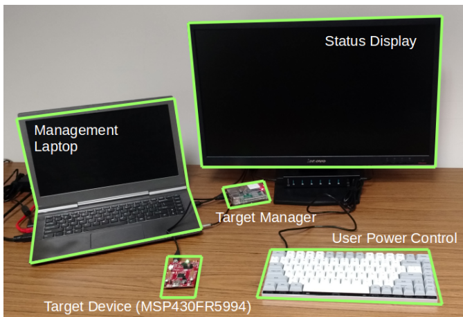
Fig. 1. Demonstration layout with components. The user power control will directly manage the power to the target device during the demonstration.
