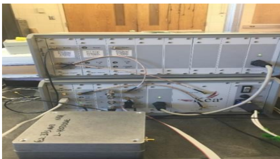
Fig.3: Kea 2 NMR Spectrometer used for pulse generation.
