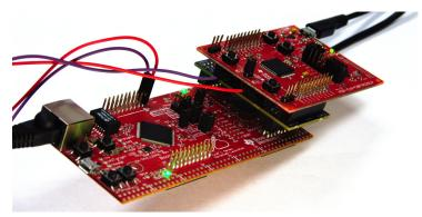
bottom, one device being benchmarked (XBD) on the top, and a power shim (XBP) in between.
