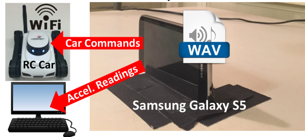
Figure 1: By playing specially crafted music on a phone, the audience will control the on-phone accelerometer that causes manipulation of a remote-controlled car.
