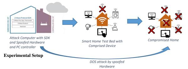
The observable demonstration will provide a pre-configured computer, along with Zniffer and PC controller dongles, and ZDP03A embedded development platform. On a monitor, reviewers will be able to see the program code, as well as the software used to view packet information, and write to the embedded system. Lastly the reviewer can test the functionality of the home network with a mobile phone connected to the IRIS Hub that is used to control the system.
